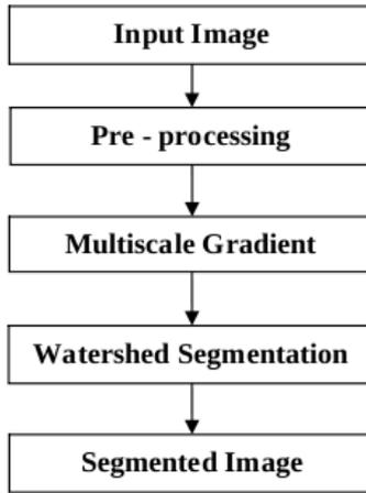
Figure 1: Block diagram of different steps
