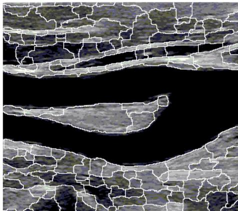
(e) Watershed segmentation on 2a after pre-processing, multiscale morphological gradient operation and removal of small minima with threshold 4.
