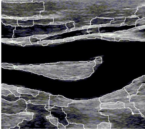
(a) Watershed segmentation on 2a after pre-processing, multiscale morphological gradient operation and removal of small minima with threshold 10.
