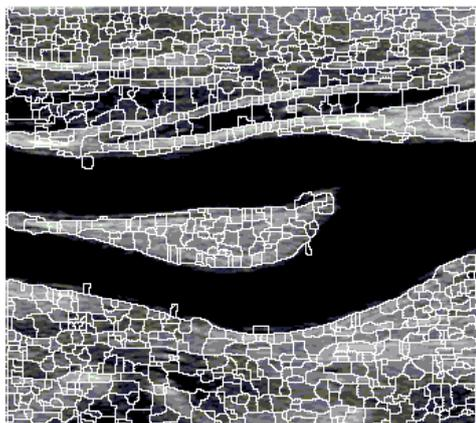
(d) Watershed segmentation on 2a after pre-processing and multiscale morphological gradient operation.
